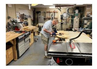
On the left is a Compound Miter Saw. In the center is a "Saw Stop" Table Saw, which detects body contact with the blade and stops instantly.
