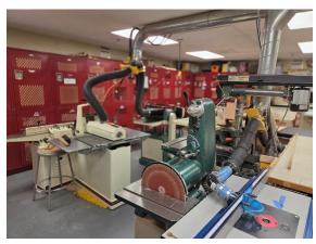
On the right side of the room are Belt and Disc Sanders, a Surface Planer, Jointer, a Radial Drill Press and a Router Table.
